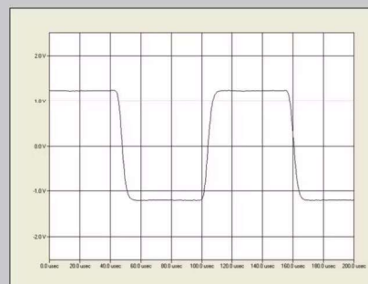
Fig.2 PrimaLuna EVO 300 Hybrid, small-signal 10kHz squarewave into 8 ohms.
