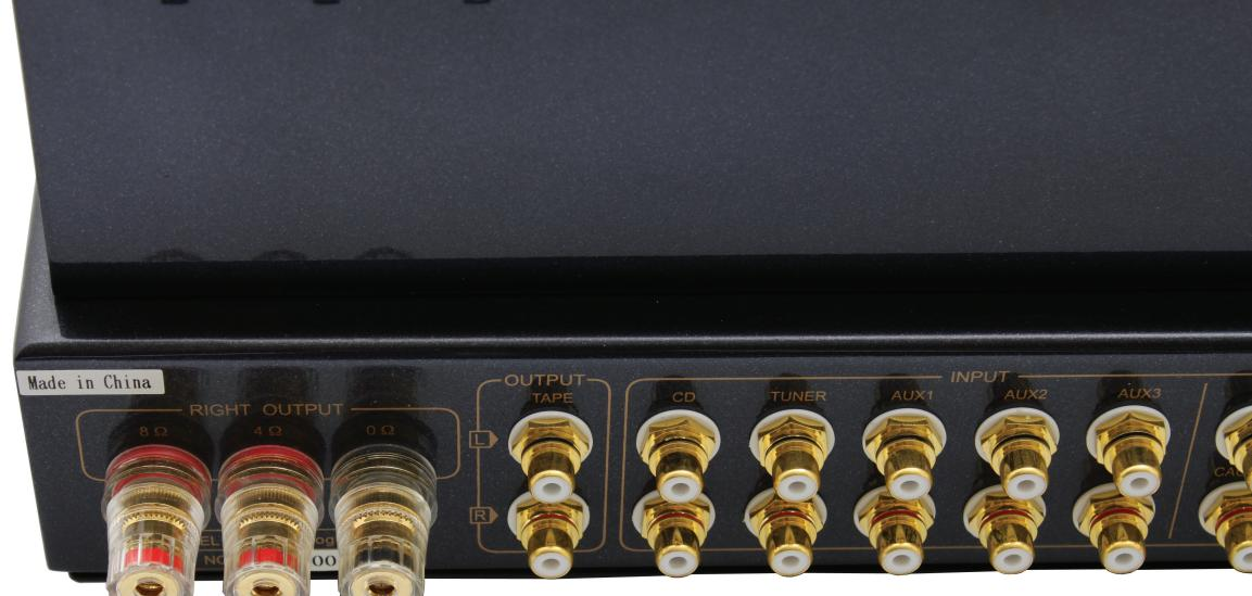
used the power cord that shipped with the DiaLogue One). The back panel also hosts the speaker terminals, and has connections for 4 Ohm or 8 Ohm speakers.
