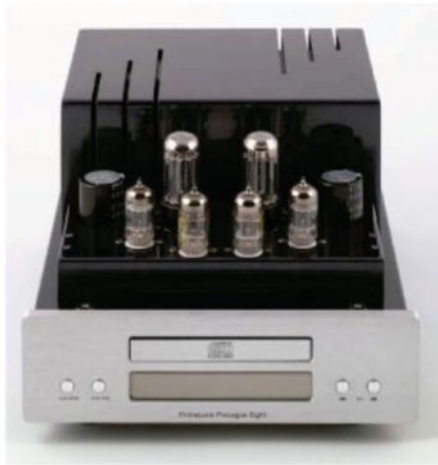
The two 5AR4 rectifier tubes sit at the back, the signal tubes at the front.
